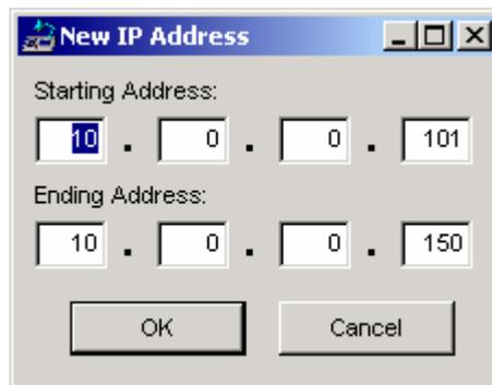
Figure 18 – Add a single IP address or address range.
